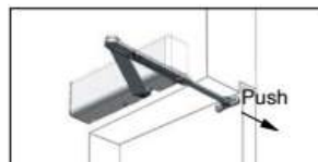
Top Jamb Installation Closer Installed Above Door On "Push" Side.
