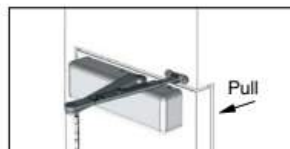
Standard Projecting Arm Installation: Closer Installed on "Pull" Side of the door
